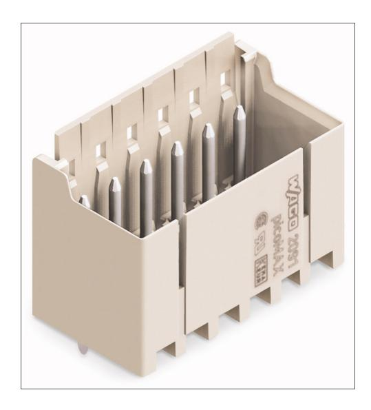
Printview: Male header with straight solder pins; 3-pole; Pin spacing 3.5 mm / 0.138 in - Item No.: 2091-1403
