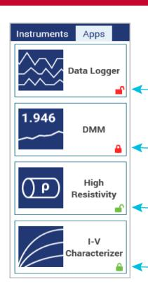
When you first open KickStart, the Instruments tab displays available instruments on the left. Select the Apps tab and you will see a lock on each App. The text below describes the licenses and lock icons:
