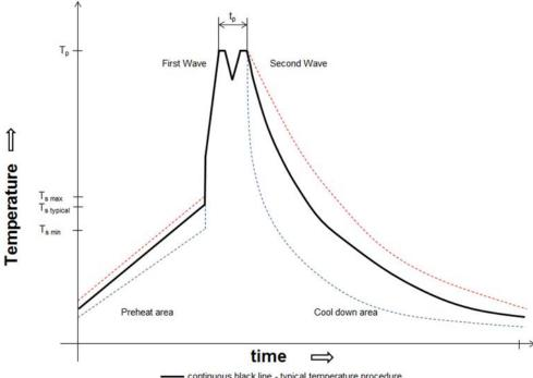
continuous black line - typical temperature procedure
