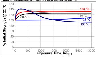
Cured for 1 week @ 22 °C Lap Shear Strength, ISO 4587: Grit Blasted Mild Steel (GBMS)
