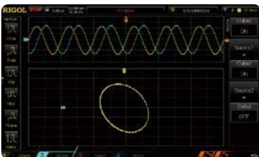
Built in 2 channel 25MHz Signal Source(MSO/ DS1000Z-S)
