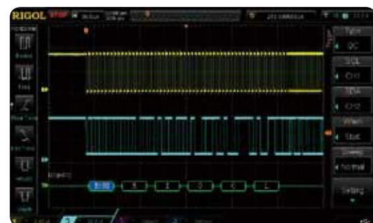
Optional Serial Bus Triggering and Decoding functions(RS232,I2C,SPI)
