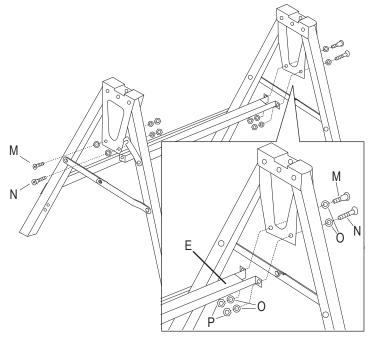
Connect the center pipe (E) to the mounting plates of both leg components. To do so, use the screws (M and N), washers (O) and nuts (P).
