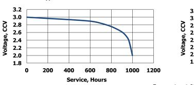
Load: 10K ohms - Continuous Typical Drain @ 2.9V: 0.29 mA
