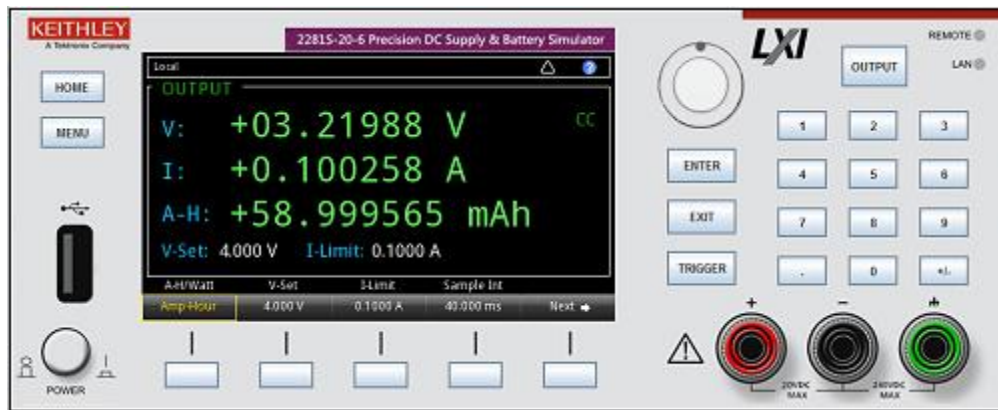
Figure 56: Virtual front panel for web page control
