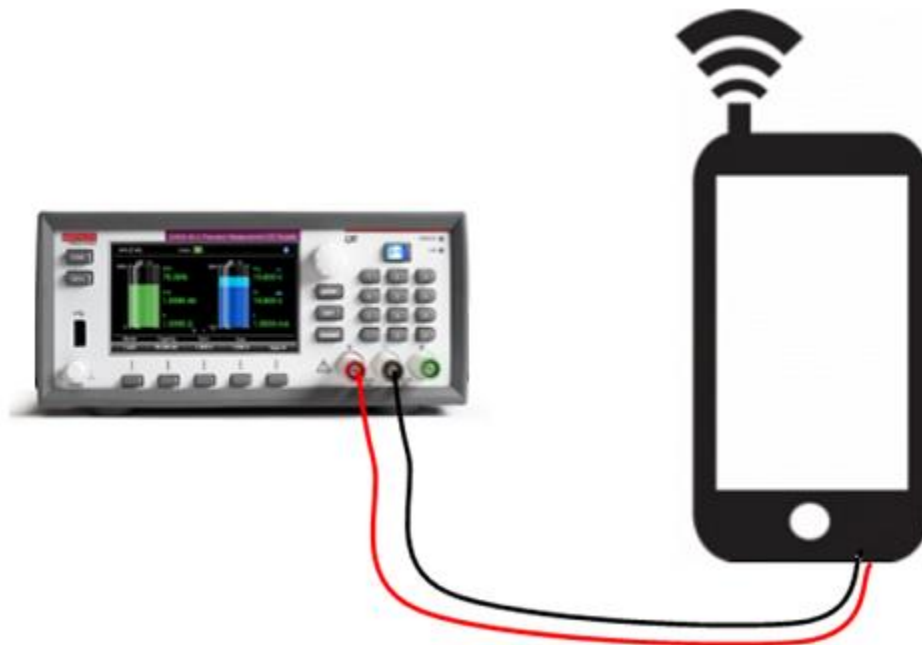
Figure 124: Battery simulation device connection
