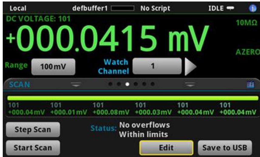
Figure 46: SCAN swipe screen - scan results
