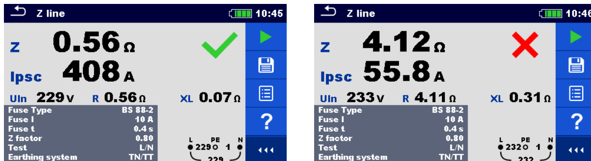
Figure 7.52: Examples of Line impedance measurement result
