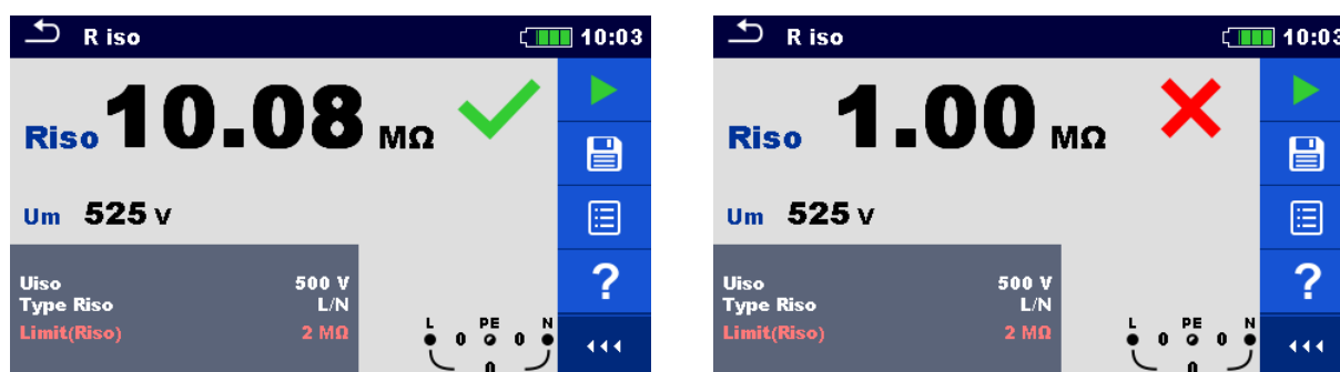
Figure 7.9: Examples of Insulation resistance measurement result
