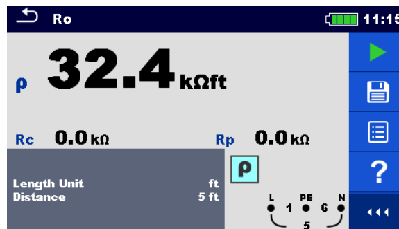
Figure 7.75: Example of Specific earth resistance measurement result
