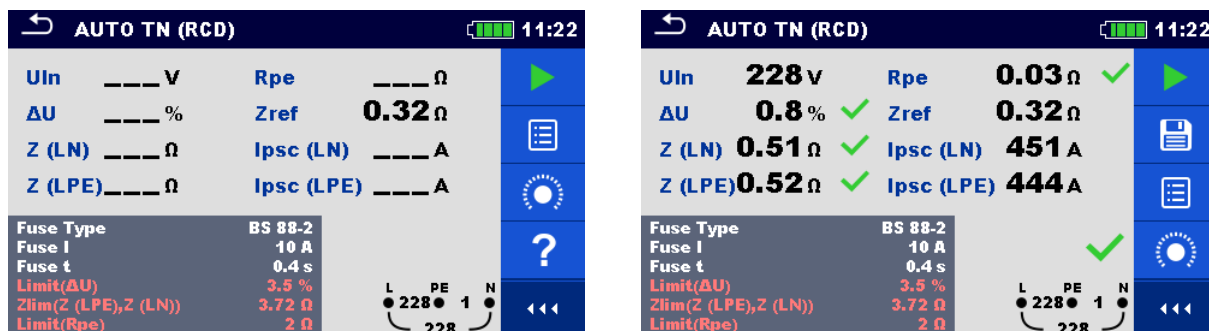
Figure 7.106: Examples of AUTO TN (RCD) measurement results
