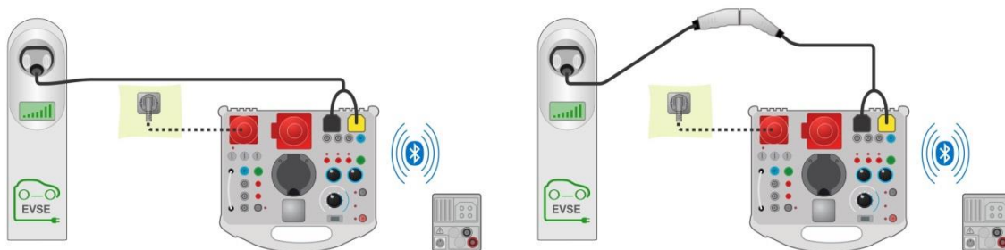
Figure 7.125: Diagnostic Test, EV simulator and Errors sub-tests - connection to EVSE
