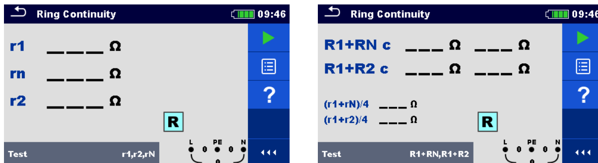
Figure 7.29: Ring continuity measurement menus
