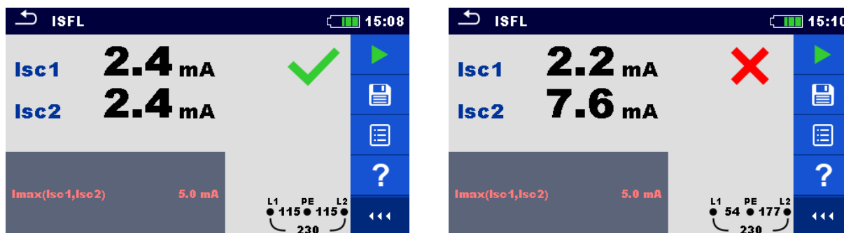
Figure 7.91: Examples of First fault leakage current measurement result
