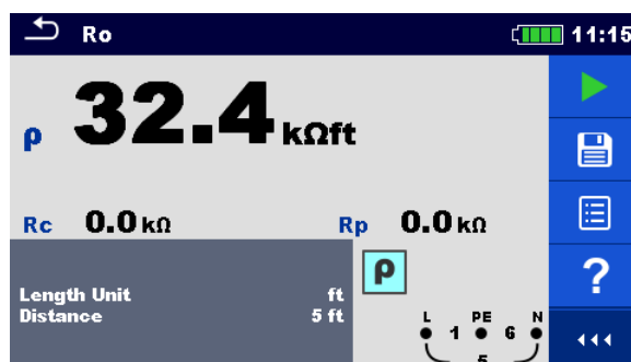
Figure 7.104: Example of Specific earth resistance measurement result
