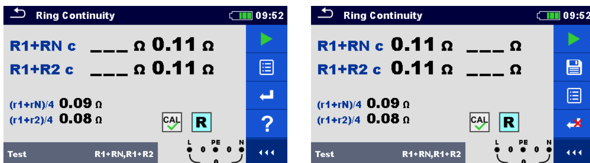
Figure 7.39: Examples of Ring Continuity measurement result
