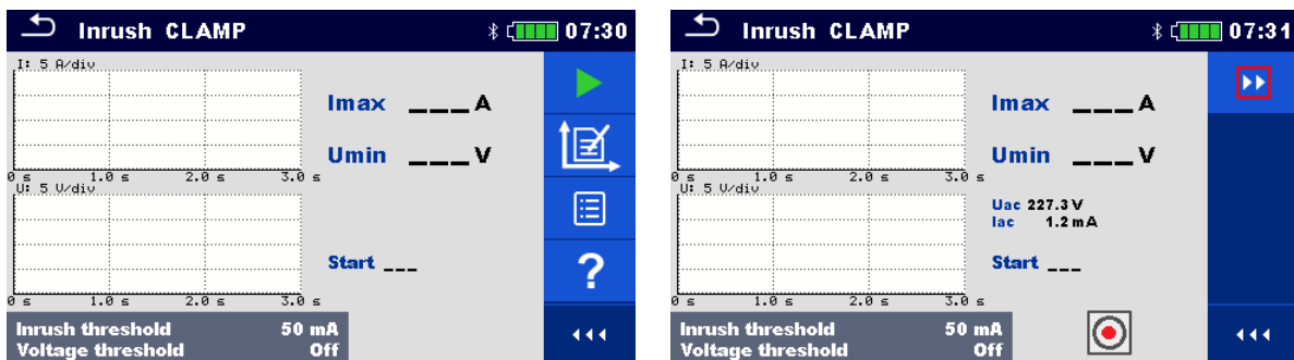
Figure 7.163: Inrush CLAMP menu – setup on the left, waiting for trigger on the right
