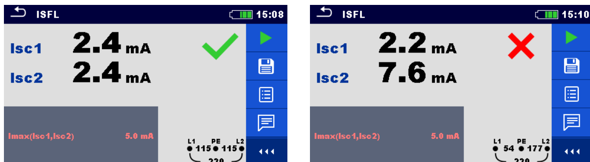
Figure 7.120: Examples of First fault leakage current measurement result
