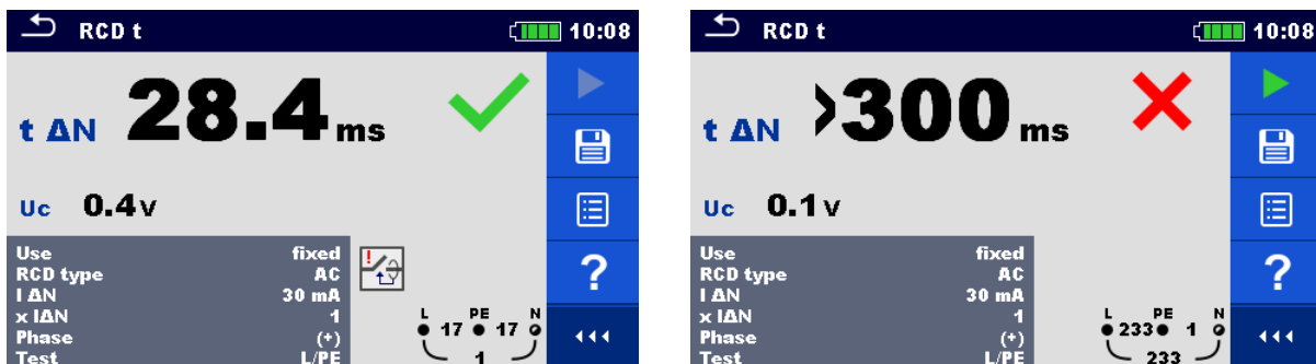
Figure 7.44: Examples of Trip-out time measurement result
