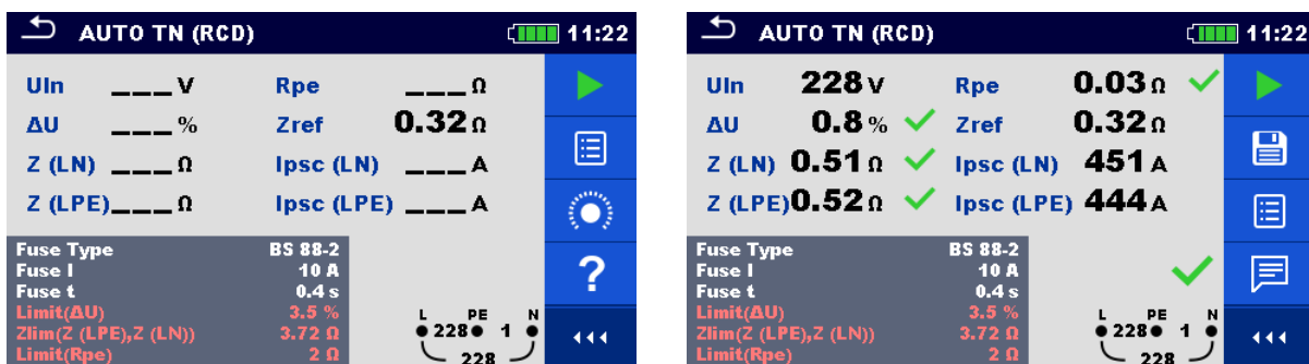
Figure 7.139: Examples of AUTO TN (RCD) measurement results
