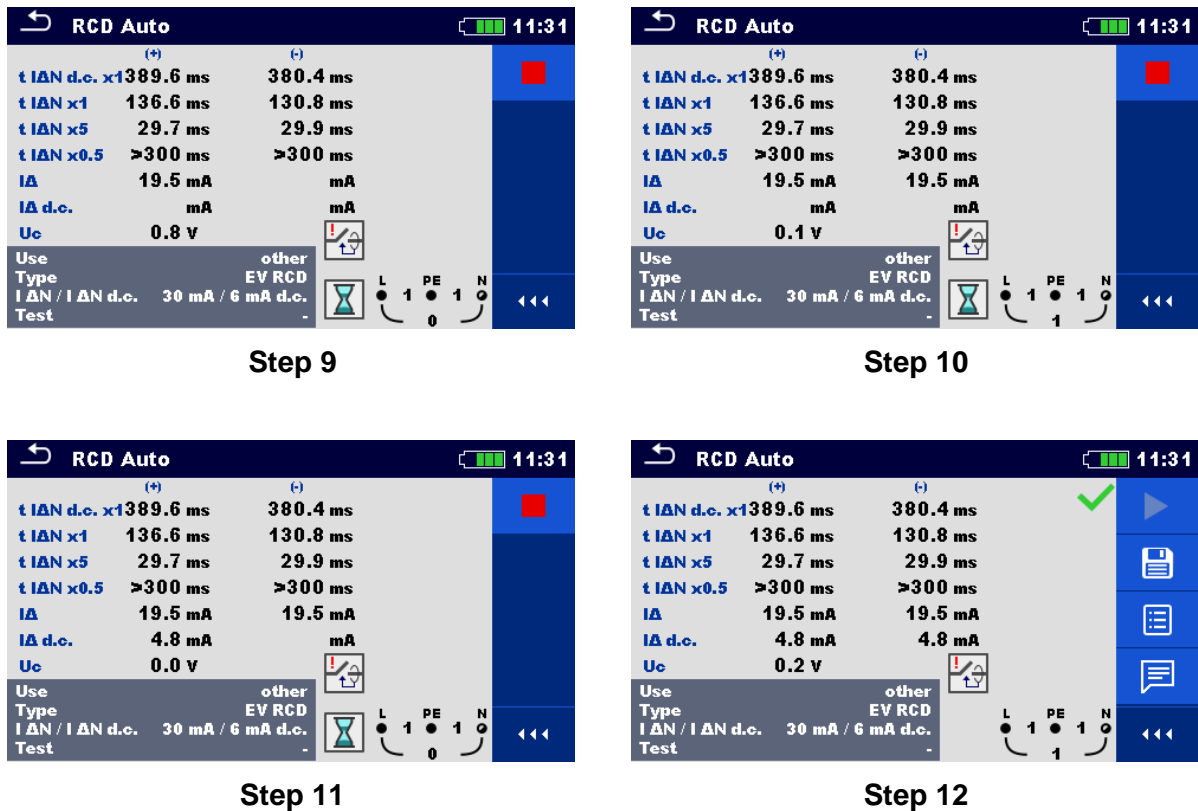
Figure 7.46: Individual steps in RCD Auto test
