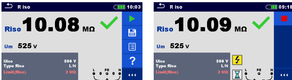
Figure 6.1: Single test screen organization, example of insulation resistance measurement
