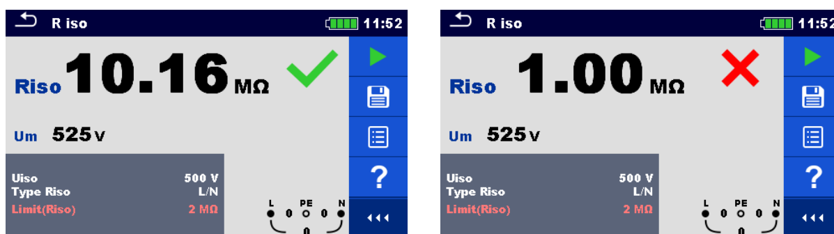
Figure 7.9: Examples of Insulation resistance measurement result
