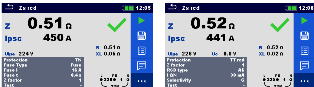
Figure 7.57: Examples of Zs rcd measurement result
