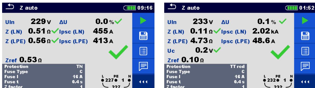
Figure 7.83: Examples of Z auto measurement results
