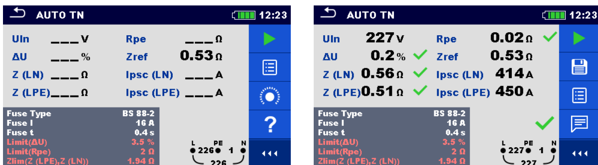
Figure 7.142: Examples of AUTO TN measurement results
