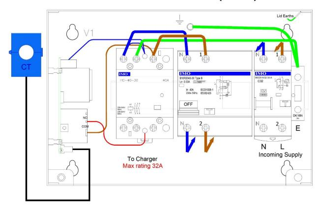
Connect the supply cable from the distribution board (or meter tails) directly to the RCBO 'Incoming Supply' terminals. Connect the outgoing cable to the contactor L, E & N terminals.
