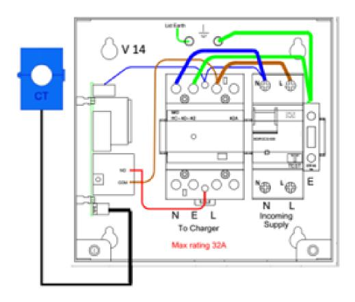
Connect the supply cable from the distribution board (or meter tails) directly to the RCBO 'Incoming Supply' terminals. Connect the outgoing cable to the contactor L, E & N terminals. If required, connect the CT to the 3 pin connector on the PCB. Check ALL power and earth connections before switching on.
