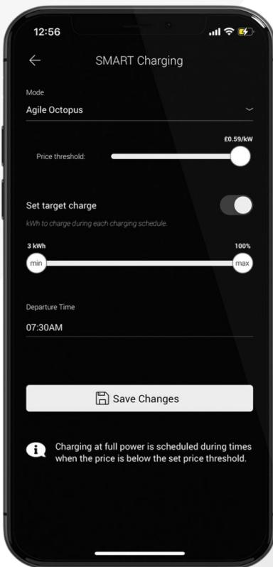
**Note** The 'Set target charge' option can be used to define how much charge you want to deliver within the set time. If the desired target charge set here cannot be achieved within the scheduled time frame, then the charger will adapt the schedule, and increase power output to ensure that it is met. Additionally you can set a departure time, to ensure that you have the charge you need, when you need it
