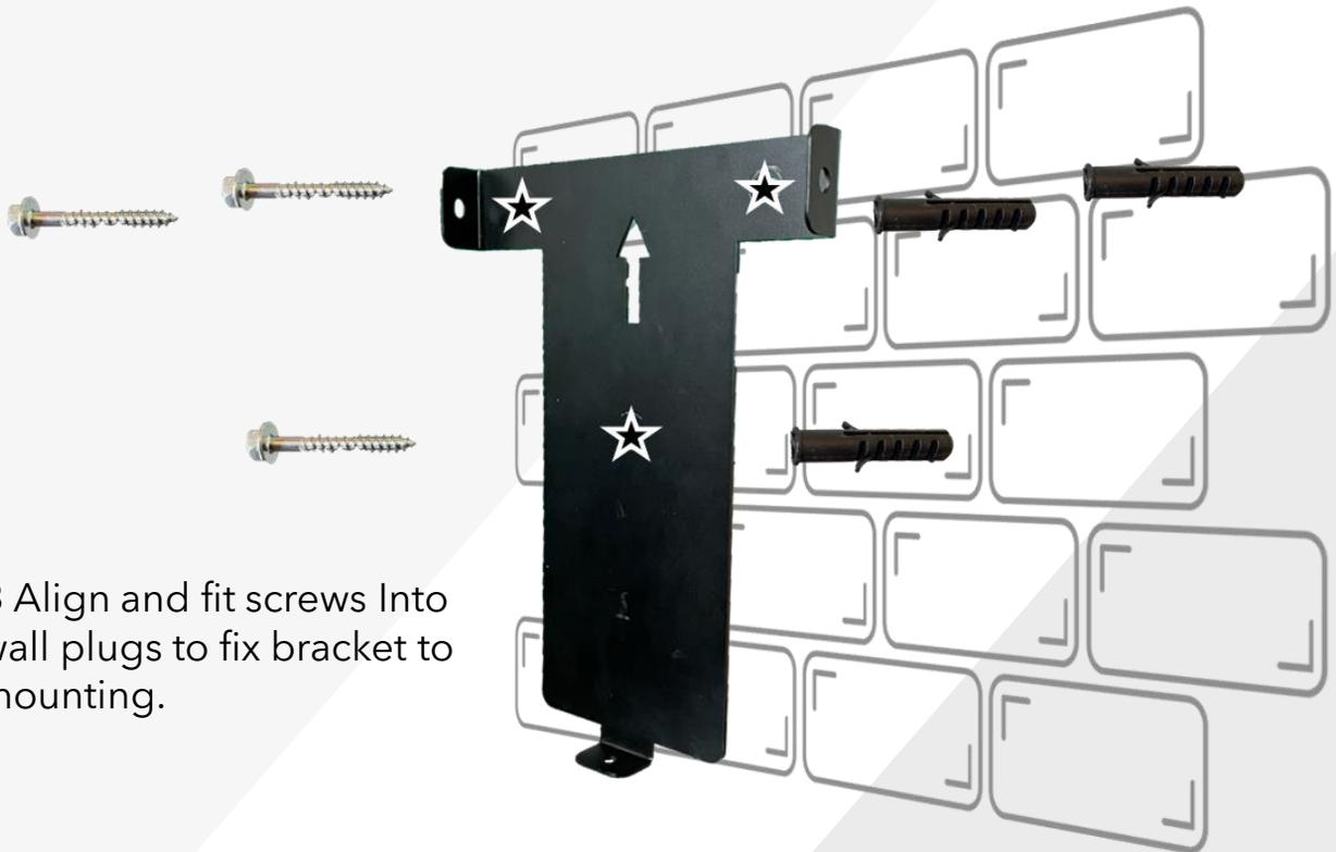
**3** Align and fit screws into wall plugs to fix bracket to mounting.
