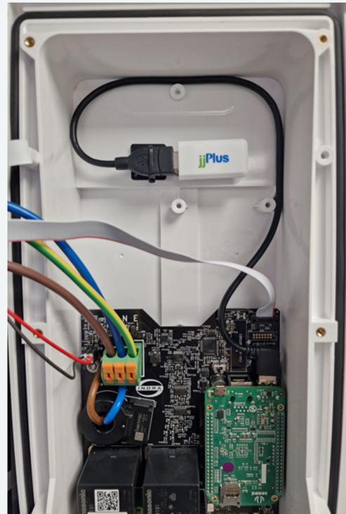
Figure 12: Smart PRO Dongle Placement
