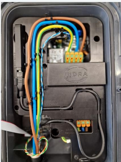
Figure 15: Smart LUX™ 4G Dongle Placement
