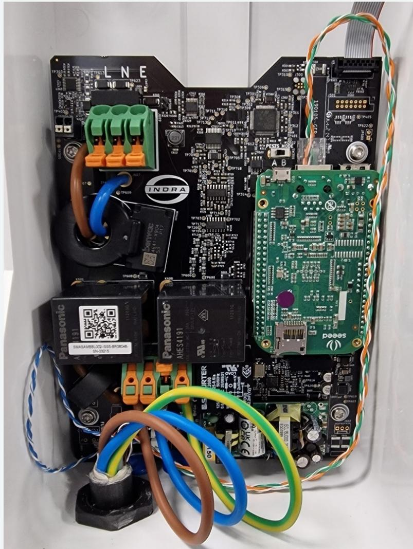
Figure 7: Smart PRO Mains Cable Routing
