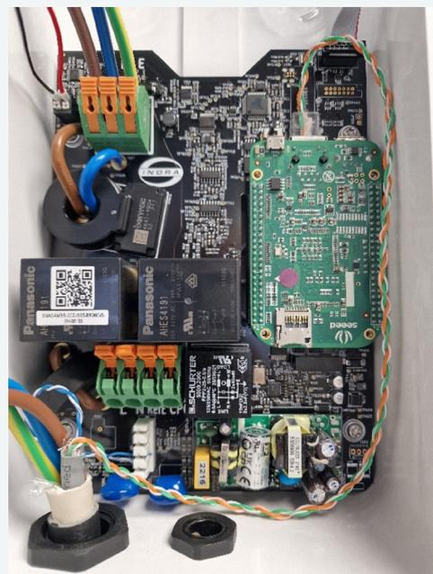
Figure 14: Smart PRO Data Cable Routing
