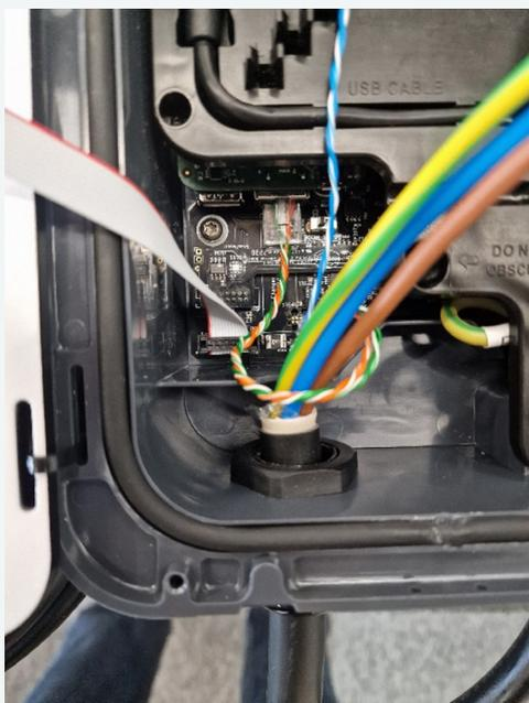
Figure 13: Smart LUX™ Data Cable Routing
