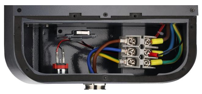
**CAUTION:** Take care not to over tighten the incoming supply PE, N and L screw terminals, to avoid damage occurring due to over tightening.
