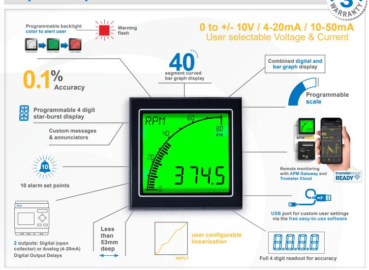
Featuring an acclaimed easy-to-read display and a versatile set of inputs, the Process Meter takes the APM into a wide range of new industrial applications.
