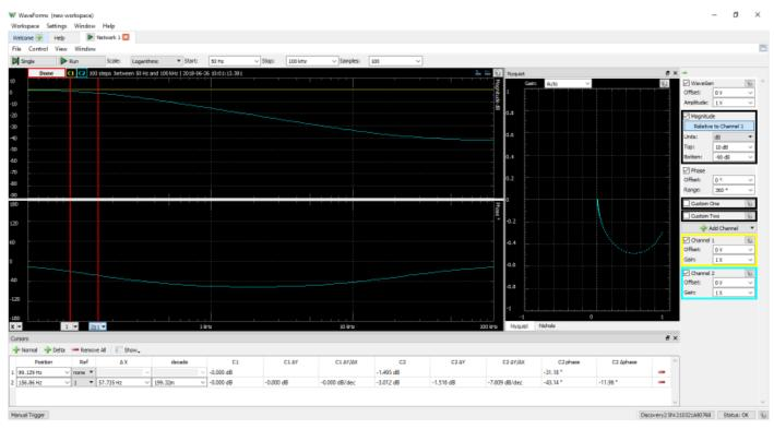
The Analog Discovery Studio can be used with WaveForms' "Network" instrument to view the amplitude and phase response of a circuit under test. Nichols and Nyquist plots can also be viewed with this instrument.
