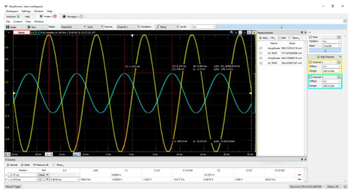
The Analog Discovery Studio can be used with WaveForms' Oscilloscope instrument to capture analog input data via the analog input ("Scope") channels, using either BNC cables or MTE cables. When this instrument is used, the Analog Discovery Studio's analog input channels act as a two-channel, 14-bit, 100 MS/s oscilloscope.
