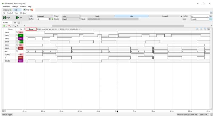
The Analog Discovery Studio can be used with WaveForms' "Logic" instrument to act as a Logic Analyzer. When used this way, the 16 digital input/output channels are configured to capture high/low logic states on connected pins at a sample rate of up to 100 MS/s. These channels are capable of interfacing with 3.3V and 1.8V logic signals, and are tolerant to voltages of up to 5V.
