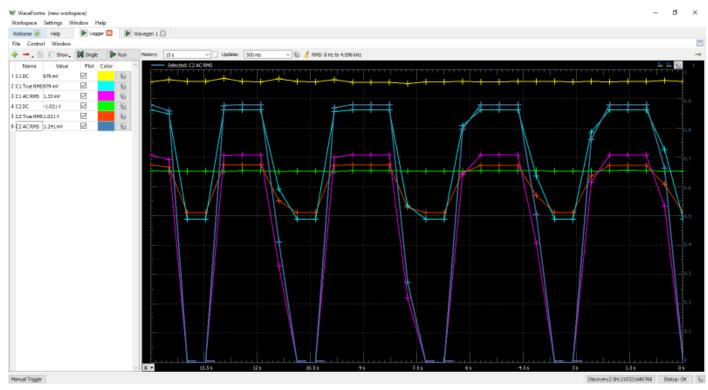
The Analog Discovery Studio can be used with WaveForms' "Logger" instrument in order to capture large buffers of analog input data on the Scope pins.
