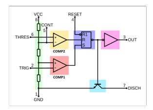
The image on the left shows a 555 silicon chip and the image on the right shows the circuit diagram of what is inside. Looking at the internal circuit diagram of the 555 timer the following can be seen:
