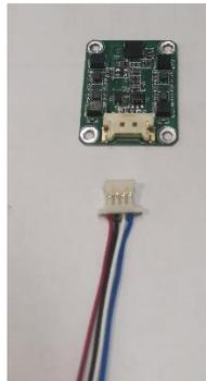
**Step 3** Refer to the following figure for wiring, and fix the 4 PIN data cable at ①②③ position by using the adhesive.
