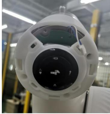
**Step 9** Install the sensor plate in the specified position on the J6 joint safe skin with M2 screws.
