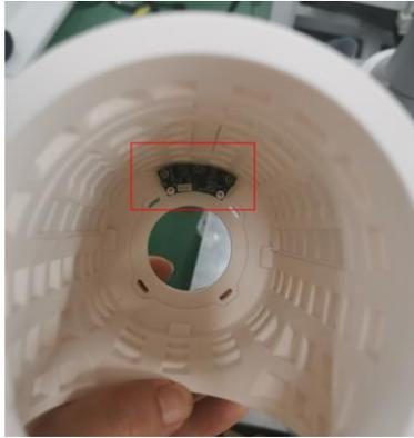
**Step 10** Install the J6 joint safe skin into the J6 joint, and install the data cable of the J6 joint on the interface of the sensor plate.
