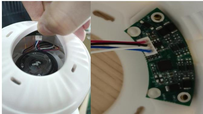
**Step 11** Tighten the safe skin of the J6 joint safe skin with M2 screws.
