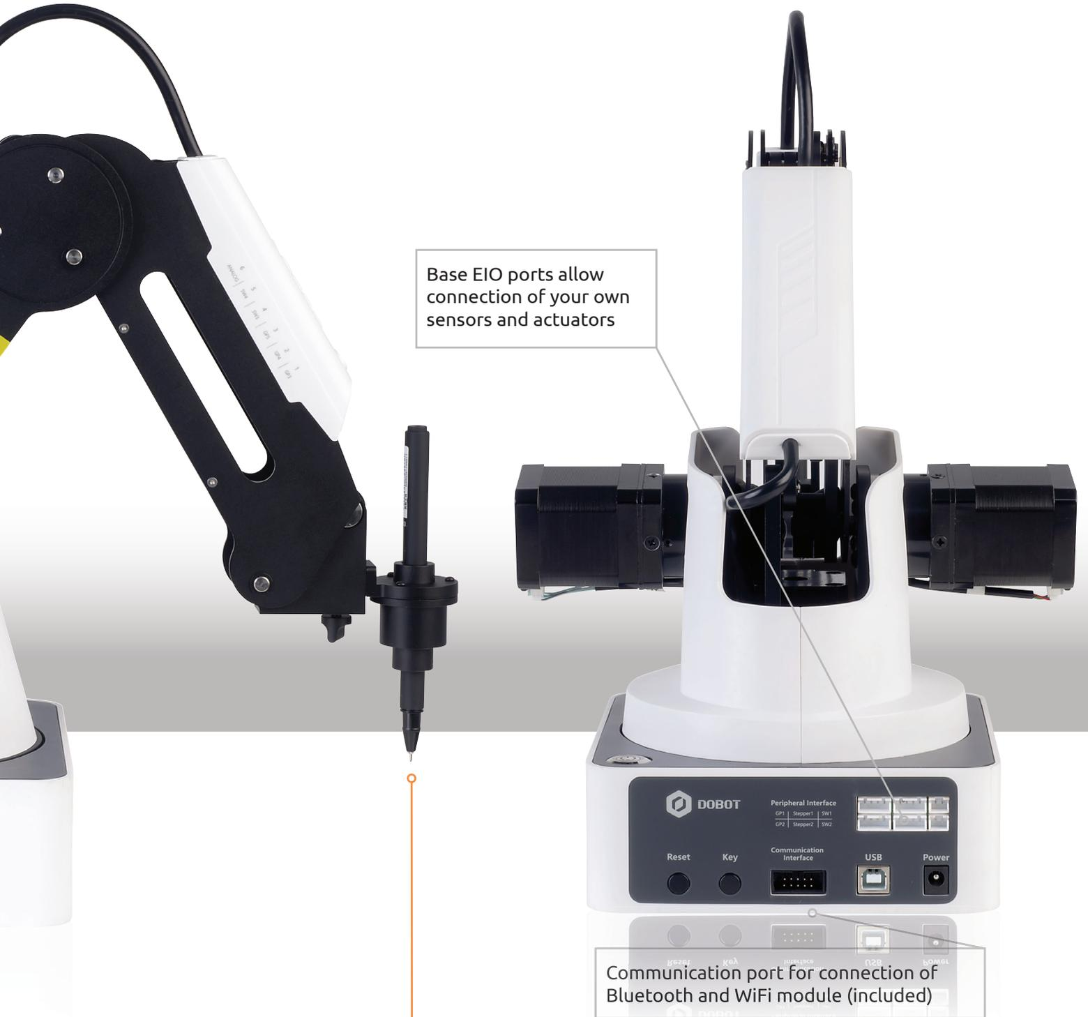
Base EIO ports allow connection of your own sensors and actuators
