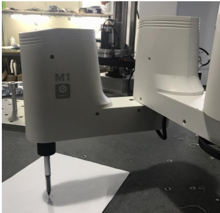
Figure 7.21 Calibration as righty hand orientation
