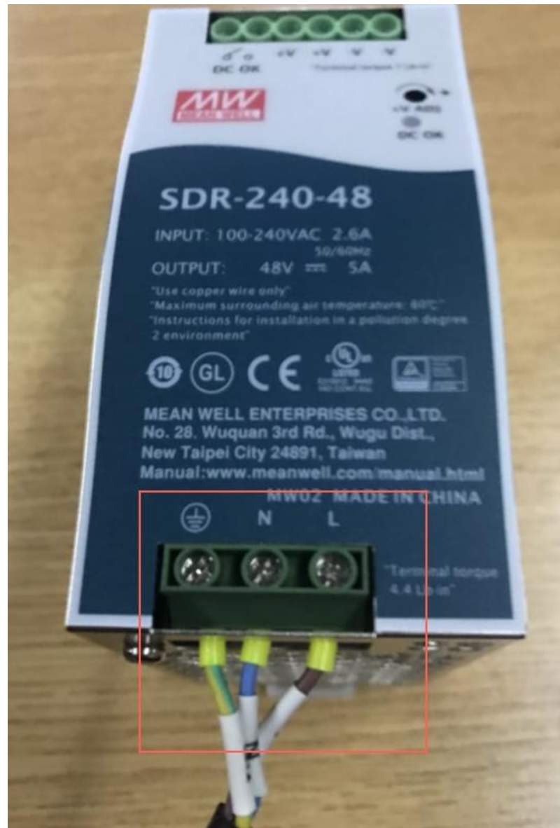
Figure 5.5 Connect power supply input cable to power adapter
