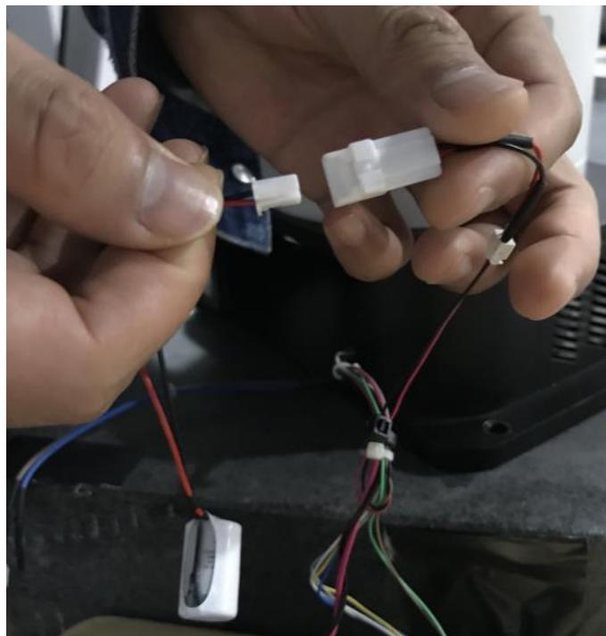
Figure 7.8 Disconnect the connector of the battery to the battery adaptor cable
