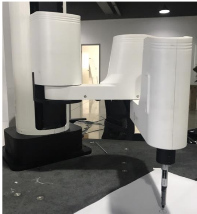
Figure 7.23 Calibration with righty hand orientation
