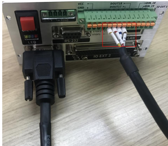
Figure 5.9 Connection between Dobot M1 and the emergency stop switch (2)
