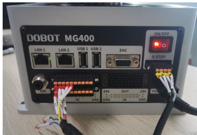
Figure 2.12 Connect gripper cable to MG400.
