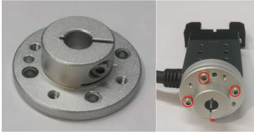
Figure 2.8 Install the end flange of MG400
