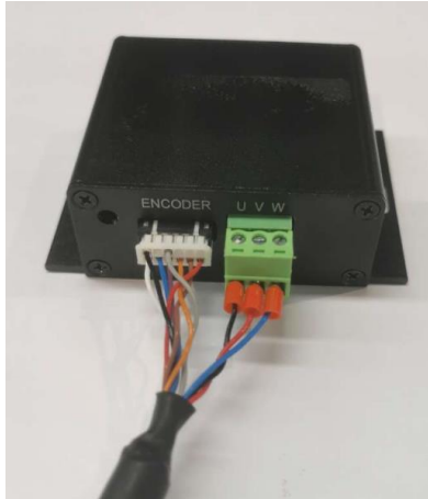
Figure 2.10 Connect servo gripper to controller
