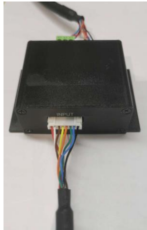
Figure 2.11 Connect gripper cable to controller
