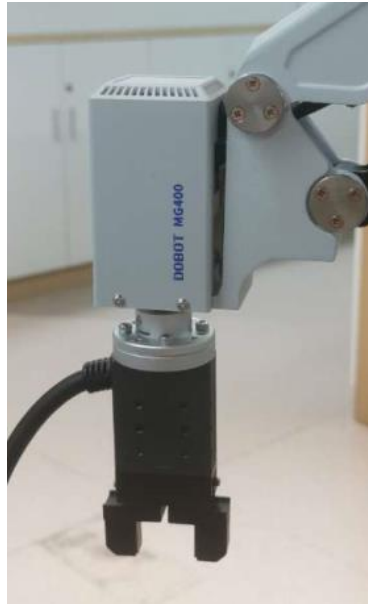
Figure 2.9 Install servo gripper
