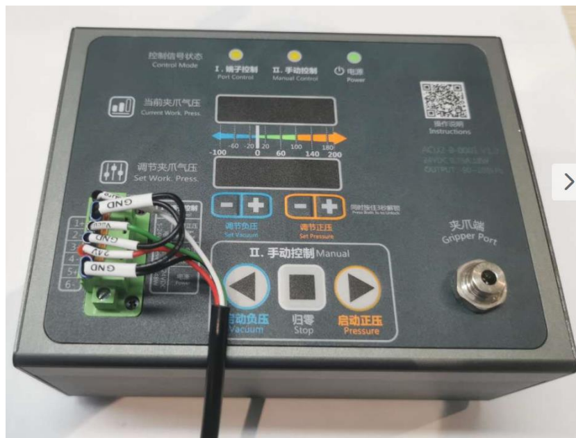
Figure 2.7 Connect gripper cable to the passive control unit
