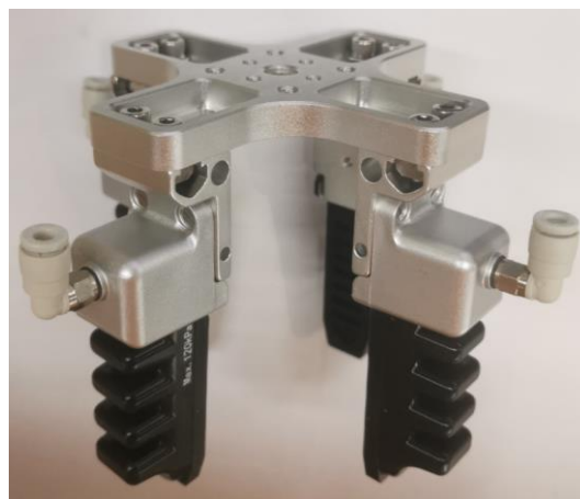
Figure 2.1 Install finger modules
