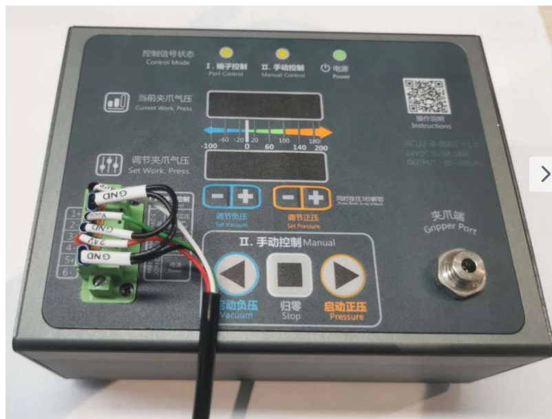
Figure 2.15 Connect gripper cable to passive control unit
