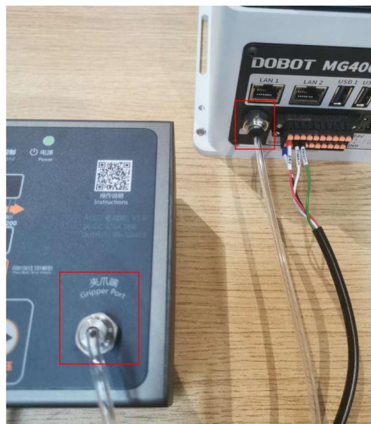
Figure 2.9 Connect PU tube
