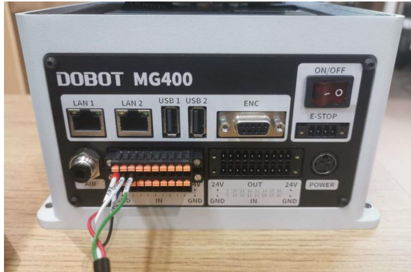
Figure 2.8 Connect gripper cable to MG400
