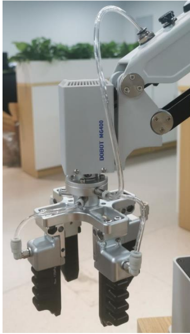
Figure 2.6 Install four-finger gripper to MG400
