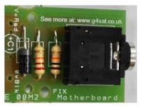
Fit them to the board as shown, this makes it easier to tuck in the capacitor.
