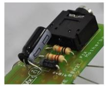
The next component to fit is the electrolytic capacitor C1. Take care to fit the short '-' lead into the hole opposite the '+'. Tuck it in carefully between the back of the download socket and to the right of R1, R2 and D1.
