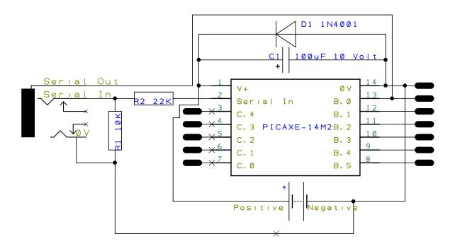
In terms of the number of components this is a fairly straightforward circuit. Access to all the I/O and +ve and –ve is provided on the two rows. Capable of 4 channels of hardware PWM and 8 bit port 'emulation' it's a handy little chip.
