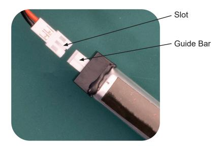
The battery **MUST** be connected with the correct orientation, as shown.
