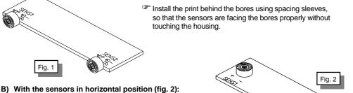
In this case the sensors are simply mounted on the print.
