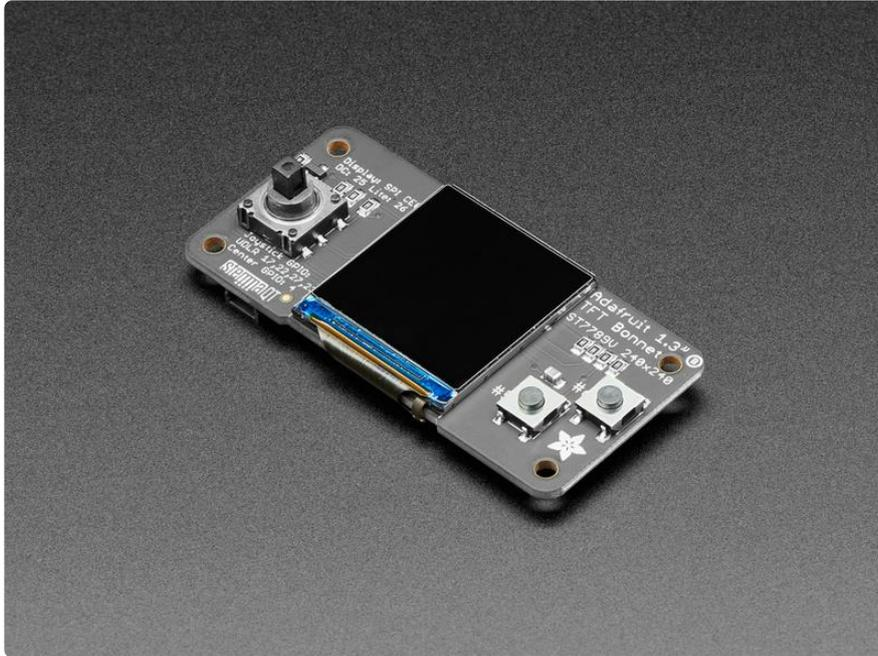
If you'd like a compact color display, with buttons and a joystick - we've got what you're looking for. The Adafruit 1.3" Color TFT Bonnet for Raspberry Pi is [the big sister to our mini PiTFT add-ons \(\)](#). This bonnet has 240x240 color pixels in an IPS TFT display, controlled over SPI. This display is super small, only about 1.3" diagonal, but since it is an IPS display, it's very readable with high contrast and visibility.
