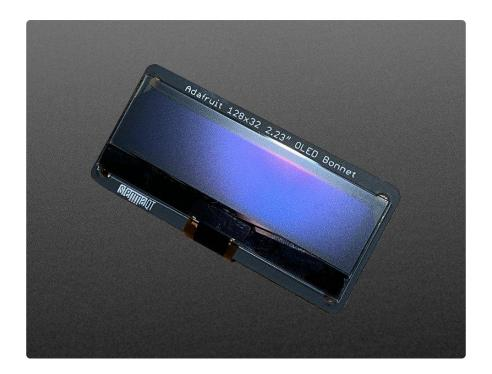
Compared to our similar PiOLED display (), this OLED has the same resolution but is much larger, so it can be read from across the room. This screen is made of 128x32 individual white OLED pixels and because the display makes its own light, no backlight is required. This reduces the power required to run the OLED and is why the display has such high contrast; we really like OLED displays for their crispness!
