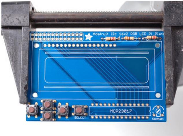
Next up we will place the buttons. These buttons are useful to send a signal to the Pi (say if you have a basic menu system). We have a 4-way 'direction pad' for up/down/left/right input and a button to the right called SELECT. These 5 buttons should be able to make 'talking' back to your project easy. These are connected to the I2C port expander chip so they require no extra pins on the Pi, our library does the work of reading whether they are pressed.
