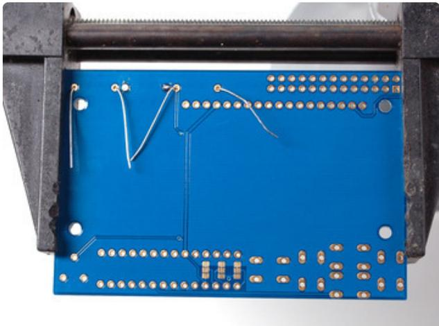
The two 220 ohm resistors **RED** and **BLUE** - named because they are the backlight series resistors for the RGB backlights on the LCDs. These resistors are colored **Red Red Brown Gold**.
