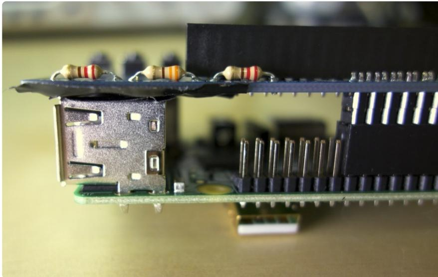
There is current limiting in the resistor circuit so it shouldn't damage the Pi if there is a short, but to be sure it is advised to cover the USB port and resistor leads in a few layers of electrical tape. Be sure to cut the resistor leads as short as possible with flush cutters and try to ensure there are no sharp edges from the cut leads or solder. See the photo below with arrows pointing to the two locations you should place electrical tape.
