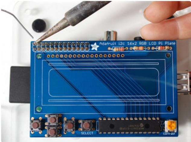
Solder in one pin, we suggest the top right, then check if the plate is sitting flat. If not, heat up the joint with one hand while stabilizing with the other until its right.
