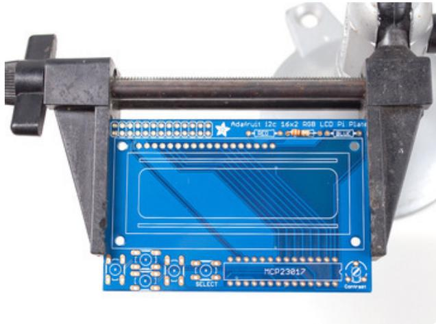
Put the printed circuit board into a vise or board holder, heat up your soldering iron and make sure you're ready to go!
