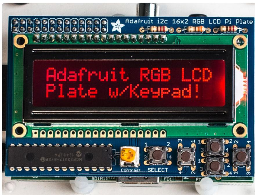
With this in mind, we wanted to make it easier for people to get these LCD into their projects so we devised a Pi plate that lets you control a **16x2 Character LCD, up to 3 backlight pins AND 5 keypad pins using only the two I2C pins on the Pi!** The best part is you don't really lose those two pins either, since you can stick i2c-based sensors, RTCs, etc and have them share the I2C bus. This is a super slick way to add a display without all the wiring hassle.
