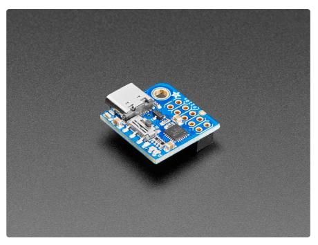
Here's another super handy add-on for your Raspberry Pi computer, perfect for 'headless' setups! The <u>PiUART</u> () adds a USB Type-C to serial connection so you can use any serial port software to connect to the Pi's console. It plugs in and is fast and easy to add whenever you need to connect to your Pi. Two LEDs connect to RX and TX on the serial converter chip so you get blinking whenever data is sent or received.
