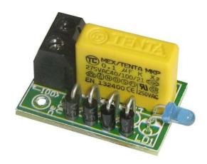
Blue LED operated on AC power-voltage Suited for mains indicator or other pilot lamps For safety guidance, stairs, corridors...
