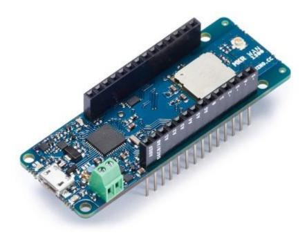
MKR WAN 1300 is a powerful board that combines the functionality of the MKR Zero and LoRa connectivity. It is the ideal solution for makers wanting to design IoT projects with minimal previous experience in networking having a low power device.
