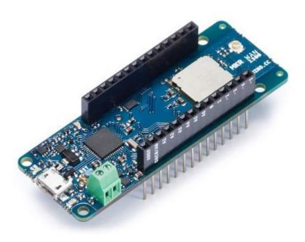
Arduino MKR GSM 1400 is a powerful board that combines the functionality of the Zero and global GSM connectivity. It is a practical and cost effective solution for makers wanting to design IoT projects with global GSM connectivity, with minimal previous experience in networking. It is based on the Atmel SAMD21 and a SARAU201 GSM module.
