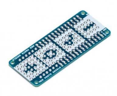
The MKR Proto Shield is a prototyping shield designed for your MKR board. This shield easily plugs onto your MKR using its provided female/male headers, and offers a duplicate breakout for each pin on the board along with many solderable through-holes on a standard 0.1" grid (2.54mm).
