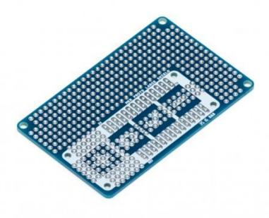
The MKR Proto Large Shield fits onto your MKR board using its provided female/male headers and enables you to fix it wherever you want with the mounting holes. This shield features a larger prototyping area with more than 300 solder points and makes connecting components to your board super simple, thanks to the silk that indicates the MKR board pins location.
