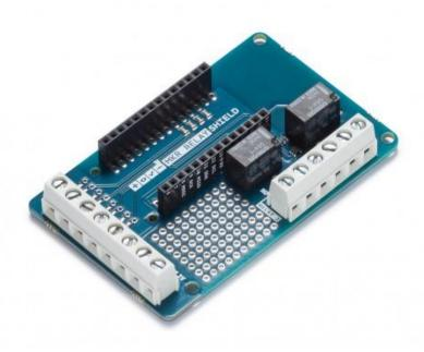
The MKR Relay Protoshield allows you to easily add relays to your MKR board based project. The shield provides two relays called RELAY1 and RELAY2 commanded by pin 1 and pin 2respectively. The shield also provides easy connection by means of screw terminal blocks to A1 to A4 analog inputs, I2C and supply voltages.
