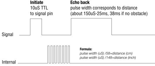
Ultrasonic Transducer will issue 8 40kHz pulse
