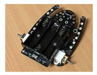
Use the 8mm countersink screws to fit the battery holder to the brass pillars.
