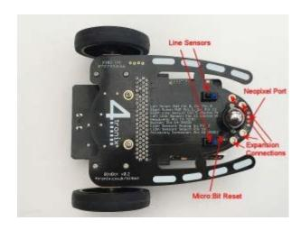
Now you can see the 2 line sensors and the port for neopixel extensions and general purpose expansion connector. Connection labelling is on the underside
