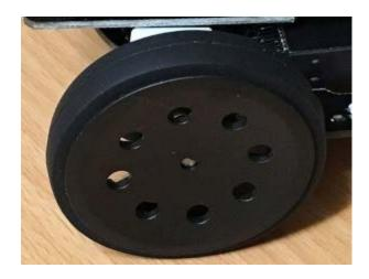
Push the wheels on, so that the axle is flush with the outside of the wheel
