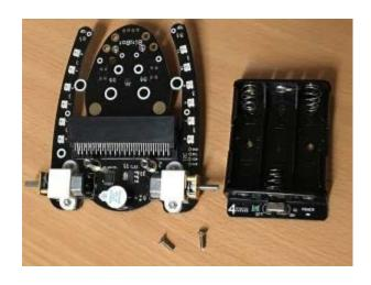
Use either 6mm panhead or 8mm countersink to fit the 12mm brass pillars to the main board (above)
