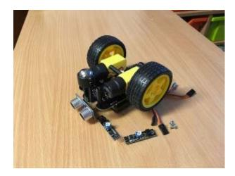
Use 2 of the 6mm M3 screws to fit a 30mm black nylon pillar to each front corner of the Robo:Bit board
