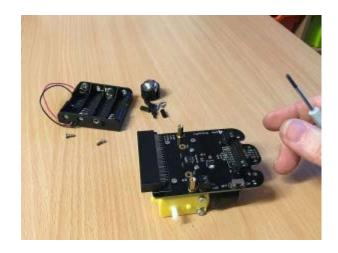
Use 2 of the 6mm M2.5 pan-head screws to attach the Robo:Bit to the upwards-facing connectors on the brass bracket assembly as shown above. Tighten securely.
