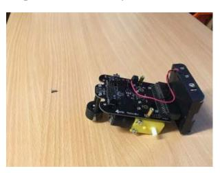
Screw the wires into the power terminal. Red to 5V and Black to GND. Wrap the wires tidily out of the way under the battery holder
