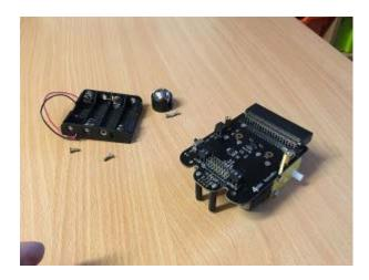
Screw each 10mm black nylon male-female pillar into a 15mm making it into a 25mm female-female pillar.
