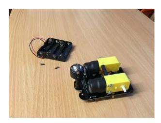
Then use two more 6mm M2.5 pan-head screws to fit the caster housing to the pillars (you will have to remove the metal ball while you do this)
