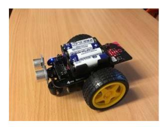
Push on the wheels. Be careful to hold the motor as the wheels can be quite stiff to fit, especially the first time
