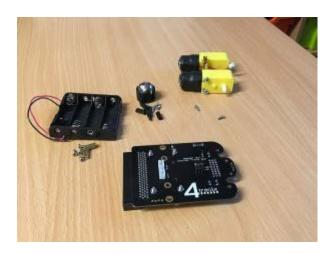
Fit 4 of the 8mm M2.5 CSK screws and the 4 nuts to the Robo:Bit as shown above. Pass each screw from the top of the board into a nut on the bottom. Tighten securely.
