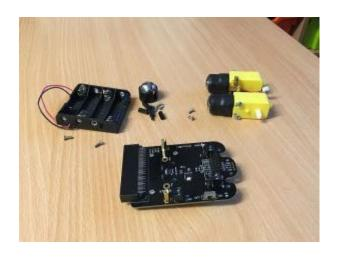
Using 2 of the 6mm M2.5 pan head screws, fit the 11mm brass pillars in place for the 4-cell battery holder – the outermost two holes – as shown above. Tighten securely
