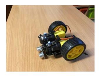
Push one of the GVS leads onto each line follower sensor. Make sure you use the colour coding: Brown for Ground (G), Red for volts (V+) and Orange for Signal (S)
