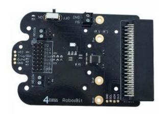
Robo:Bit is a general purpose robotics controller for the BBC Micro:Bit, that also converts easily into a self-contained little buggy.
