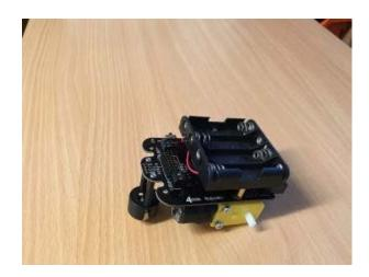
Use the remaining 2 of the 8mm M2.5 CSK (or 6mm pan head) screws to screw the battery holder to the brass mounting pillars. With some battery holders, the wide countersunk screws don't fit, so swap them with the 2 smaller pan-head screws used to hold the mounting pillars for the front caster
