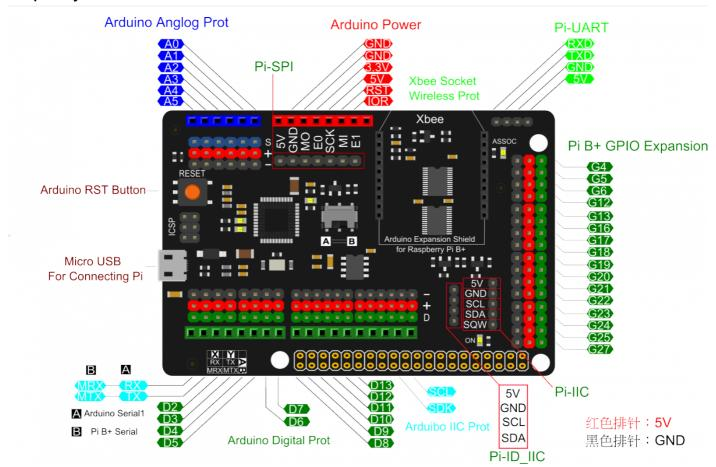
**NOTE**: The ID-I2C is an EEPROM interface, which is dedicated to connect to external EEPROM, it will test automatically EEPROM devices attached to it when it starts, is used for configuring GPIO and Linux drivers. In theory, it can be used as an ordinary I2C.
