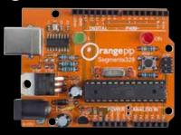
The Segments328 board is a build it yourself board designed to help students understand and appreciate the workings of a microcontroller development board.
