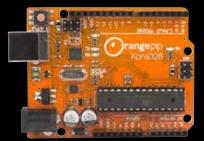
The Kona328 is a high quality Arduino UNO compatible board based on the ATmega328.
