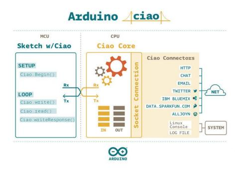
Arduino Ciao is an easy-to-use and powerful technology that enables Arduino sketches to communicate intuitively with the "outside World". It aims to simplify interaction between microcontroller and Linino OS, allowing a variety of connections with most common protocols, third-party services and social networks.
