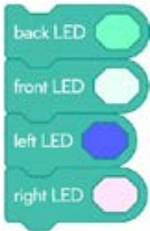
**LED Blocks:** Change the color of the front, back, left, and right LEDs. Set this using the color wheel and brightness slider, or the exact RGB (red, green, blue) values, from 0 to 255.
