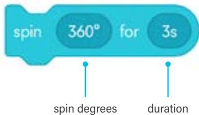
The **speed block** makes BOLT+ roll forward at speed 100. It will continue rolling at this speed until it is told to stop. The **spin block** makes BOLT+ rotate  $360^\circ$  over a duration of 3 seconds. The combination of rolling while spinning makes BOLT+ trace a circle. After BOLT+ finishes executing the **spin block**, the **stop block** sets the speed to 0.
