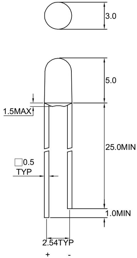
Note : 1.All dimension are in millimeter tolerance is  $\pm 0.25\text{mm}$  unless otherwise noted.
