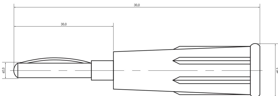
2mm Plug with special design for the spring part ensuring a reliable connection.
