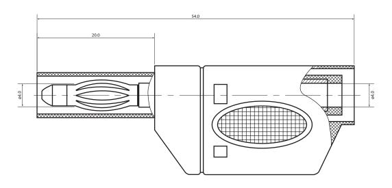
Stackable 4mm safety plug with a rigid insulating sleeve for self-assembly of test lead.
