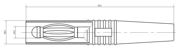
4mm Safety plug with a straight body for self-assembly of test lead.
