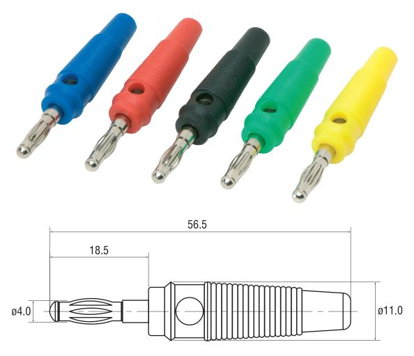
4mm Plug with the caged spring and tapering sleeve providing protection against kinking for self-assembly of test lead.
