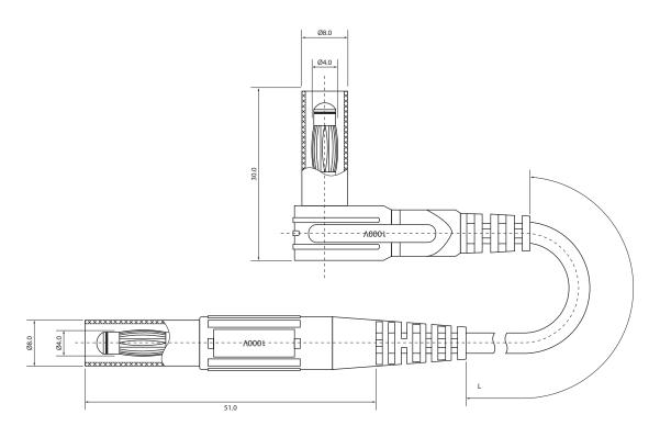
Flexible safety test lead with two 4mm straight plug and right angled plug.
