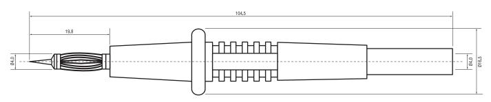
4mm Test probe with caged spring and 4mm socket at the other side
